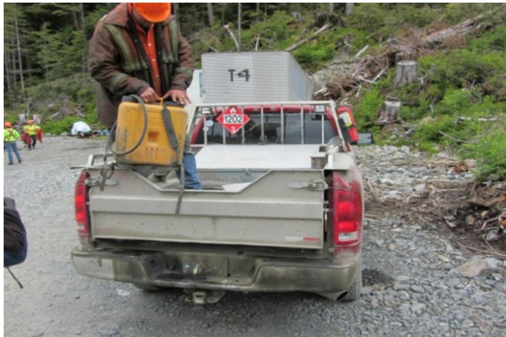
And whether a fire suppression system is ready to be used should a fire occur. In this case because the tank is empty and the nearest water supply is over 2 km away – the suppression system is not adequate.
