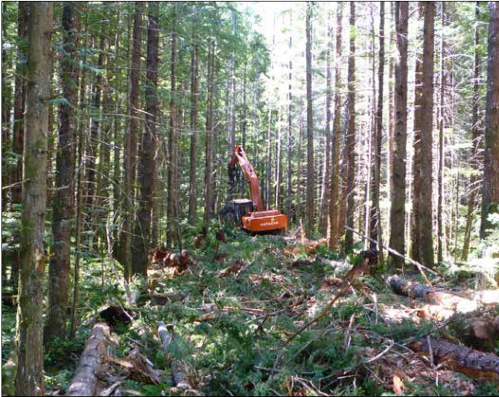
Excavator falling and processing wood in one of the thinning corridors to create a herringbone pattern to reduce “wind throw”.
